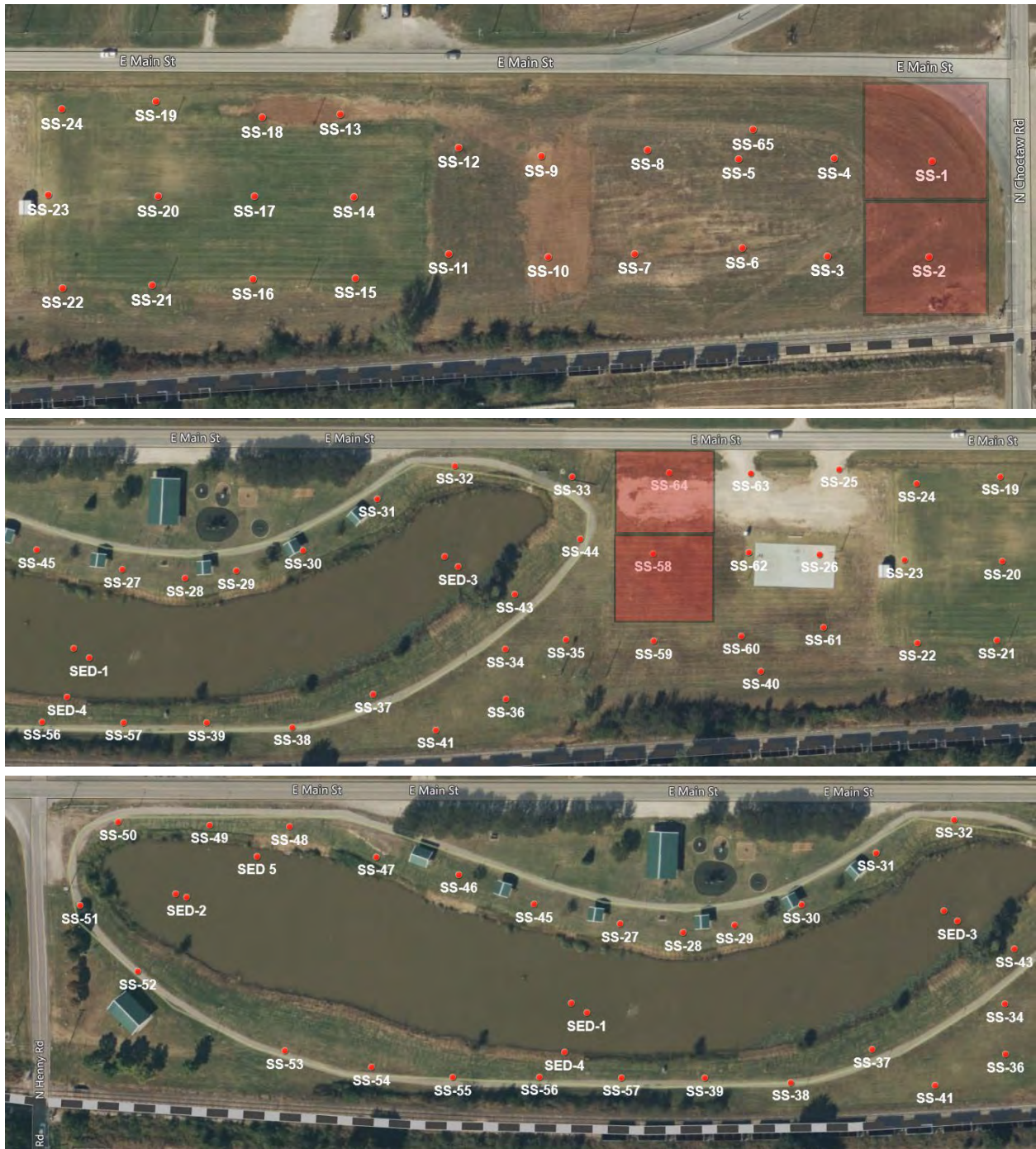
Figure 2: Soil sampling locations. Highlighted grids indicate sample result over 200 mg/kg.
